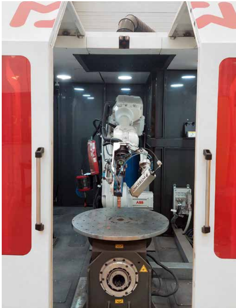
Fig. 8 The MetalWorm robotic wire-arc Directed Energy Deposition machine is designed to enhance efficiency and flexibility in metal manufacturing. With low buy-to-fly ratios, these machines minimise waste by precisely depositing material only where needed, enabling the efficient use of high-value metals (Courtesy MetalWorm)
